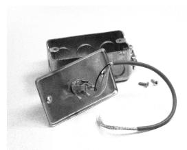
The splice point should stay inside the junction box. That is, you want to feed the long run of cable into the box rather than pulling the pigtail out. Electro-Mech provides a strain relief on one side of the junction box to secure the cable. You may choose to connect conduit directly to the junction box, in which case the strain relief will not be needed. The junction box is designed to accept 3/4-inch conduit fittings.
